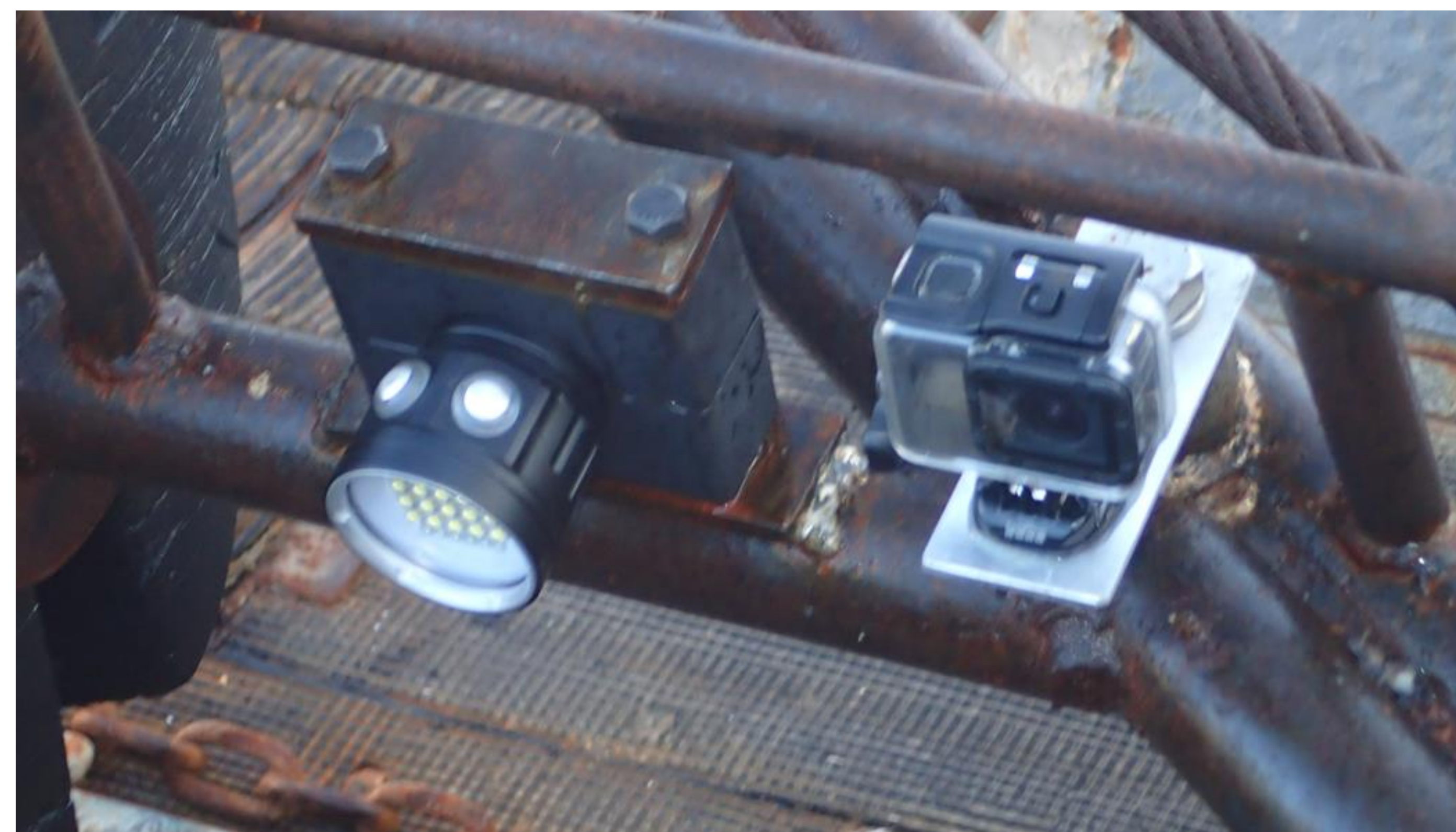
Figure 2. Image of the GoPro camera system fixed to the survey dredge
